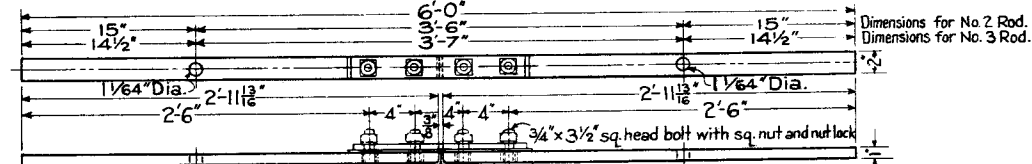
NOS. 2 & 3 SWITCH RODS (Insulated)
