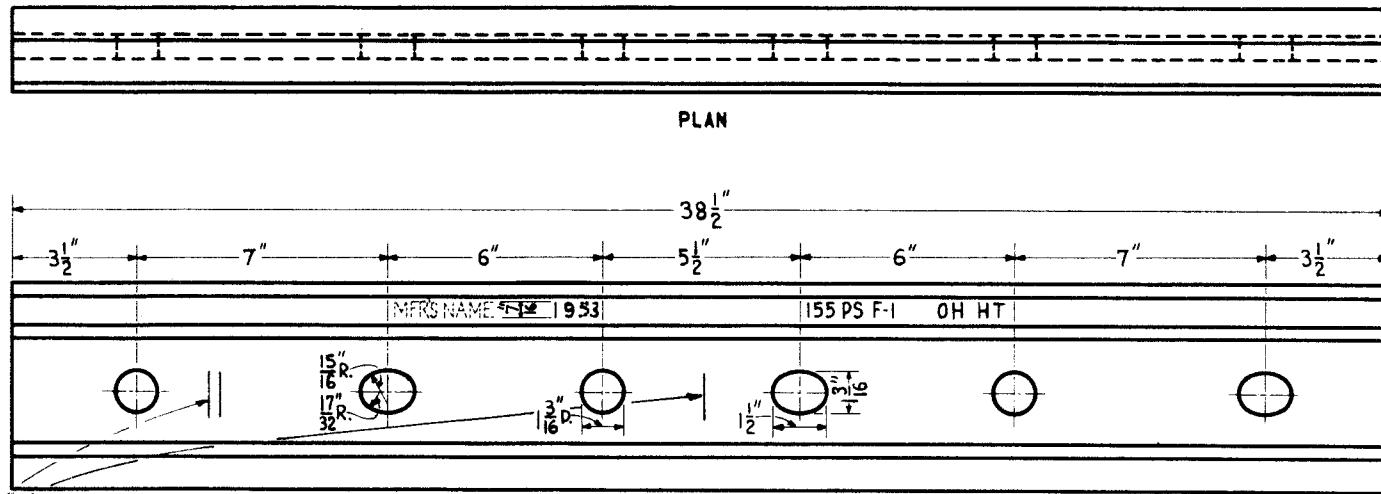
The amount of increase in fishing height shall be marked by deeply cut characters not less than  $\frac{1}{16}$ " high on outside of web in position as shown.
