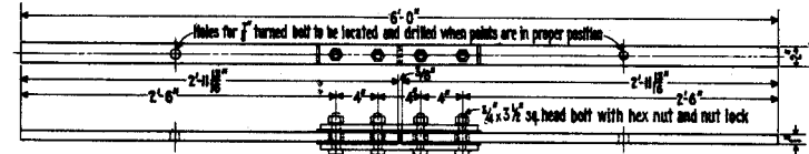
ROD NO. 2 FOR SLIP CROSSING (Insulated)
