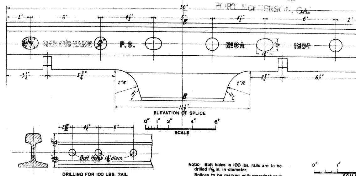
Note:- Bolt holes in 100 lbs. rails are to be drilled  $1\frac{1}{8}$  in. in diameter.
