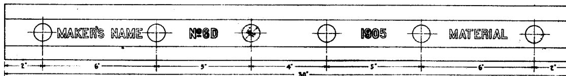
ELEVATION OF SPLICE BAR FOR 85 LBS. RAILS
