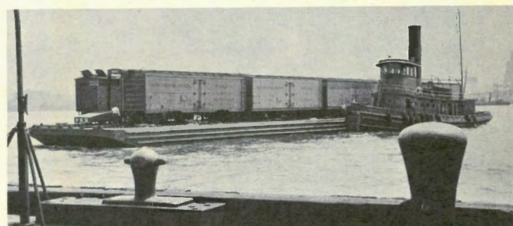
ONE OF PENNSYLVANIA'S fleet of 70 modern steel carfloats with loaded cars aboard, being transported across the Hudson River.
