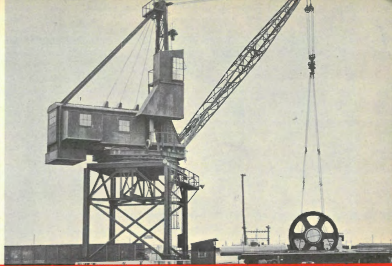
MARGINAL CRANE , capacity 65 tons, used in the transfer of excessive weight shipments between cars and lighters at Greenville.
