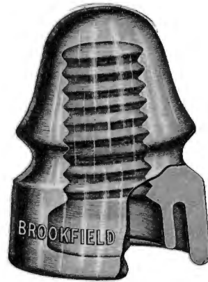
Fig. 10. DEEP GROOVE, DOUBLE PETTICOAT GLASS INSULATOR. Section removed to show inside petticoat.
