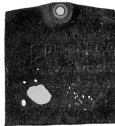
Fig. 12. APPEARANCE OF ZINC PLATE WHEN NEARLY EXHAUSTED. BSCO Cell.
