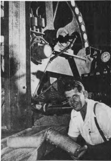
Die wheel in which sawdust is screw-compressed into Pres-to-Logs. The logs appear as circles in the outer rim of the wheel.
