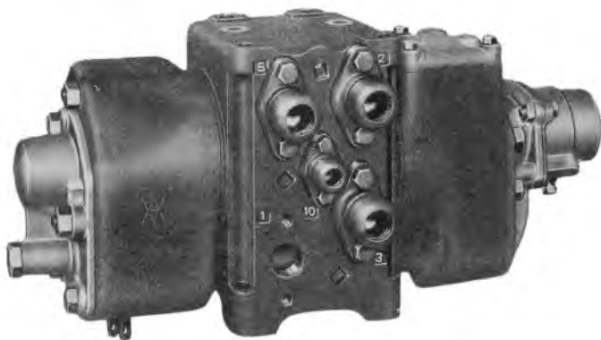
Fig. 2. View of the "AB" Valve showing the Pipe Connections
