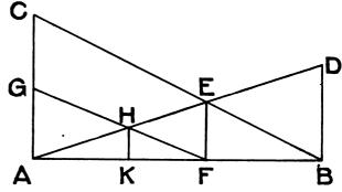
ber of branches. It is apparent that although a diagram of six lines is necessary for two resistances, each additional branch of the circuit necessitates the drawing of only two extra lines, while the arithmetical solution of the problem becomes more and more complicated as the number of branches increases.
