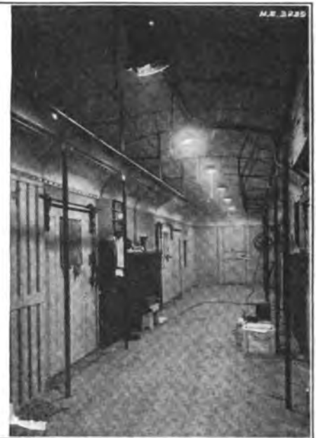
Fig. 3. Showing the Illumination with 8 ft. 6 in. Spacing which is Recommended for B-60 Cars. Note the Shadow Lines Are but Slightly More Pronounced than in Fig. 2.
