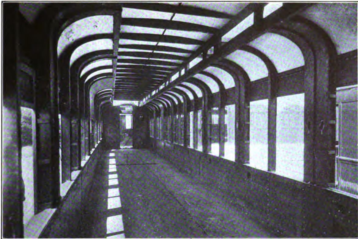
VIEW OF FRAMING FOR SLEEPING CAR.
