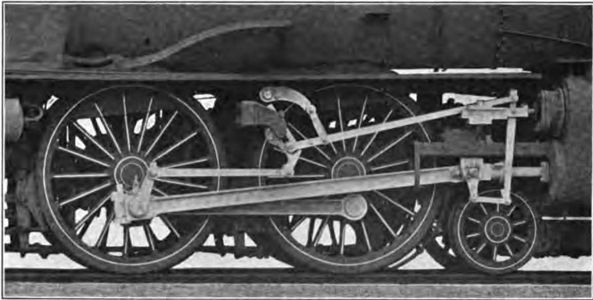
VIEW OF WALSCHAERT VALVE GEAR AS APPLIED TO CLASS E3D LOCOMOTIVE—PENNSYLVANIA RAILROAD.
