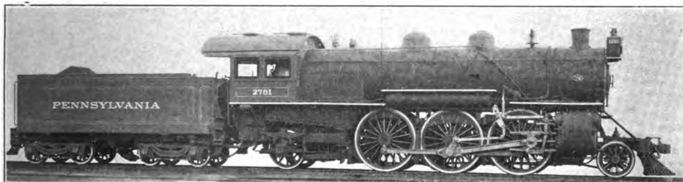
PRAIRIE (2-6-2) TYPE PASSENGER LOCOMOTIVE, WITH WALSCHAERT VALVE GEAR—PENNSYLVANIA RAILROAD.
