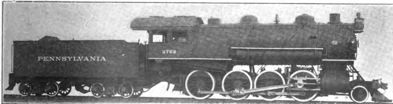
CONSOLIDATION (2-8-0 TYPE) FREIGHT LOCOMOTIVE—PENNSYLVANIA RAILROAD.
