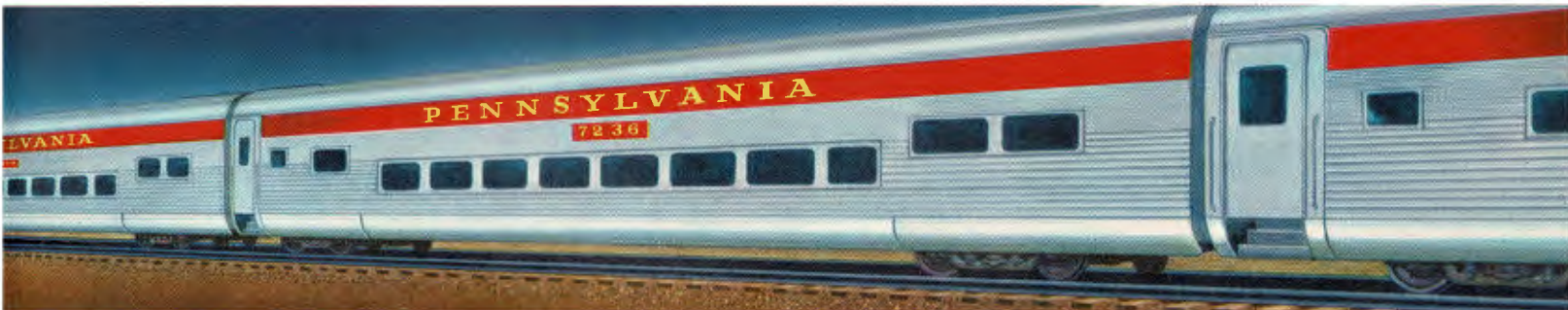
New, tubular GLIDER design for coach and Pullman cars allows their use with existing diesel and electric locomotives.
